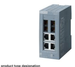
SCALANCE XB004-2 unmanaged Industrial Ethernet Switch for 10/100 Mbit/s; for setting up small star and line topologies; LED diagnostics, IP20, 24V DC power supply, with 4x 10/100 Mbit/s twisted pair ports with RJ45 sockets; 2x 100 Mbit/s multimode glass FOC port with SC socket; Manual available as a download
